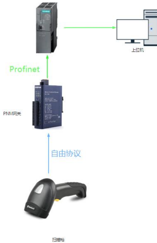
Topology of free port transparent mode
