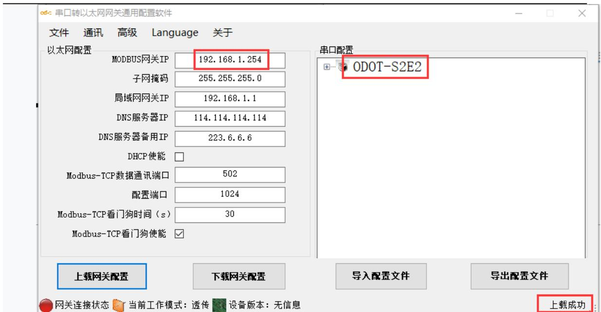
Modify the gateway IP address of the configuration software interface to:
