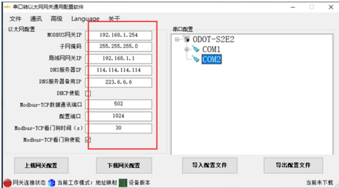
Figure 3.37 Configure gateway Ethernet parameters
