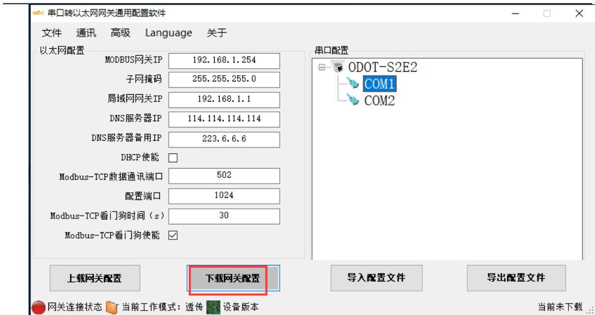
Figure 3.22 Download the gateway configuration.
