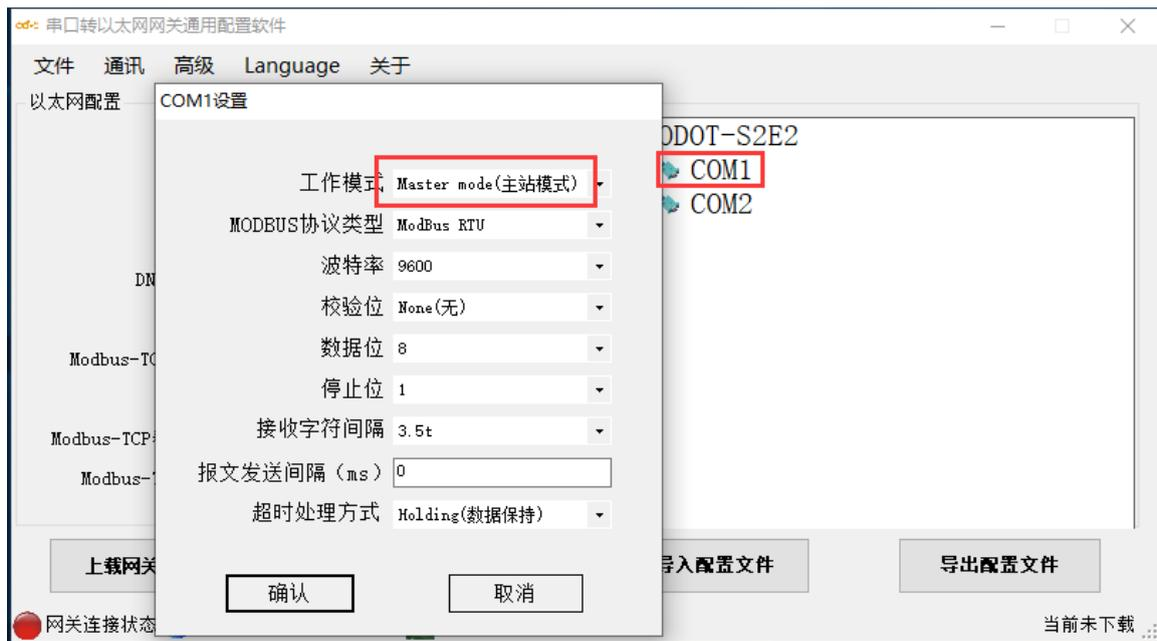
Figure 3.33 Set serial port parameters as Modbus RTU/ACII master station
