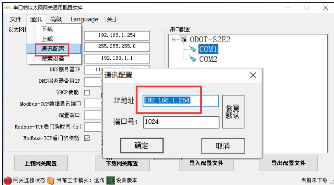
Figure 3.21 Software and gateway communication configuration
