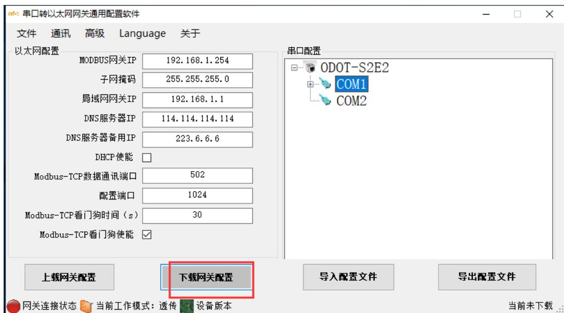
**Figure 3.8 Download gateway configuration**
