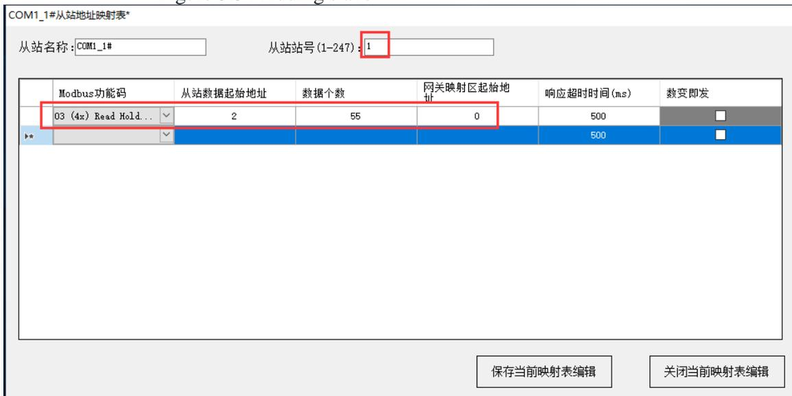
Figure 3.35 Configure slave address mapping table
