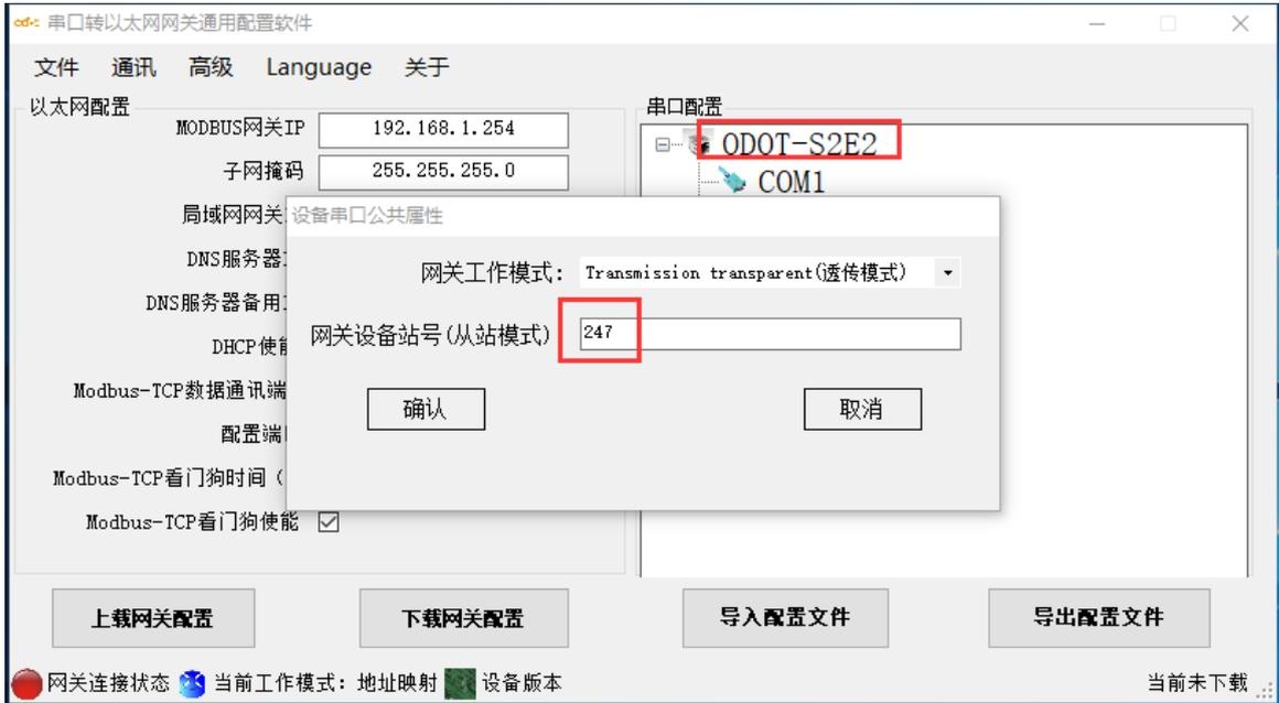
Figure 3.18 Set gateway working mode
