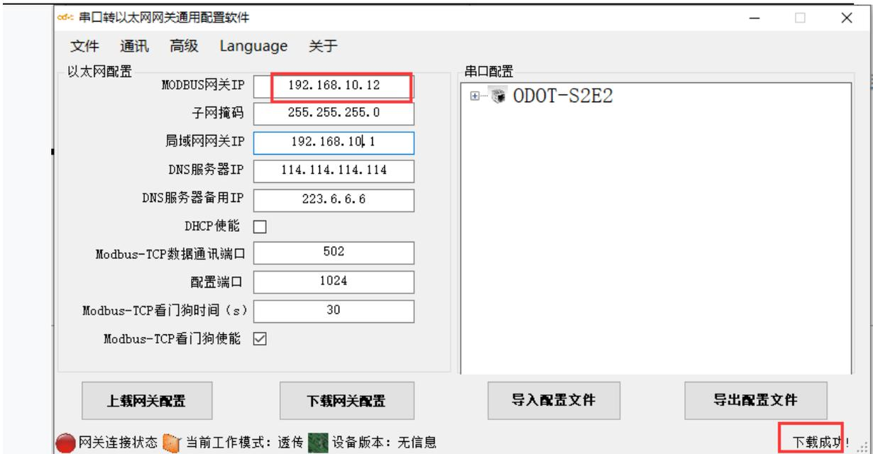
After the IP address is successfully modified, you need to change the computer's IP address to: 192.168.10.\* network segment.
