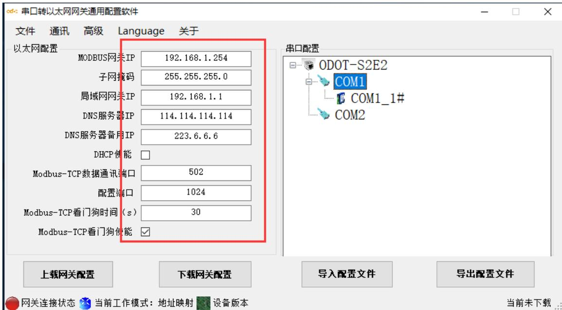
Figure 3.14 Configure gateway Ethernet parameters
