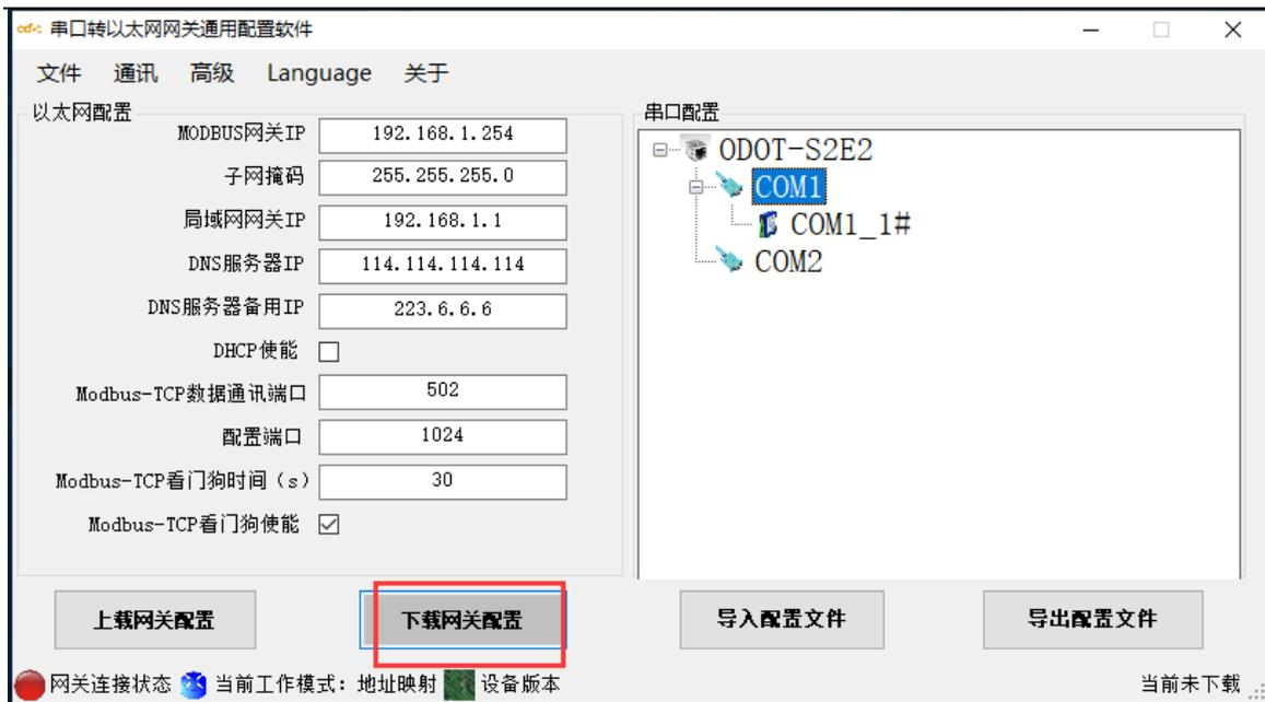
Figure 3.15 Download gateway configurations
