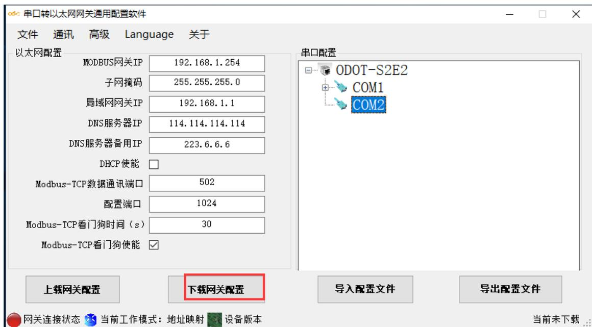
Figure 3.39 Download gateway configuration
