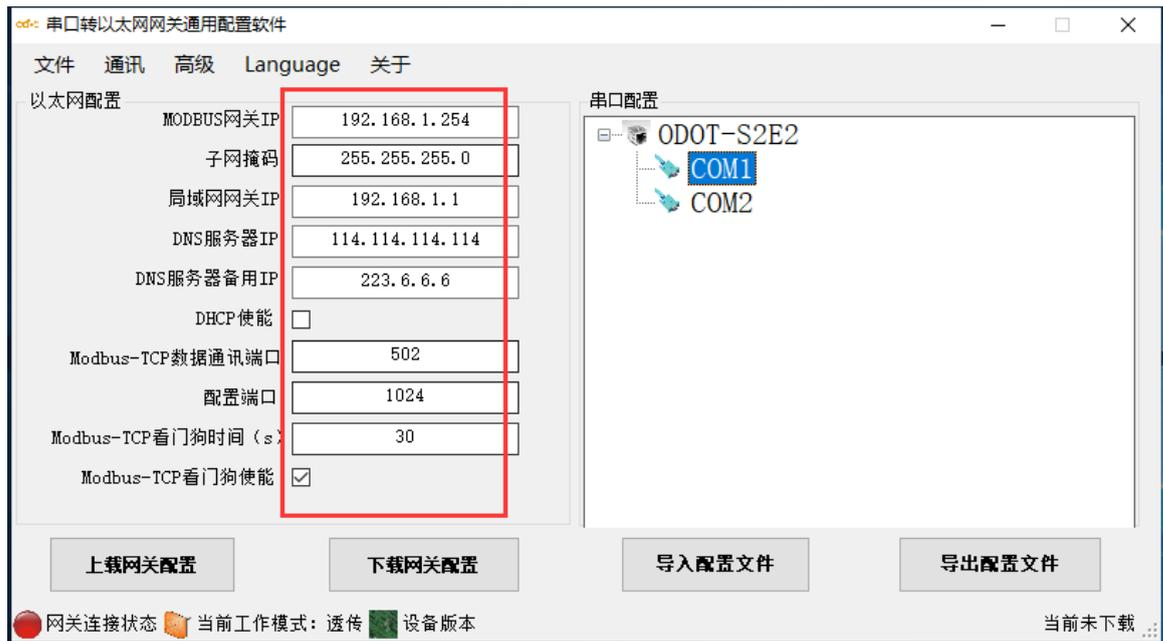
Figure 3.20 Configure gateway Ethernet parameters
