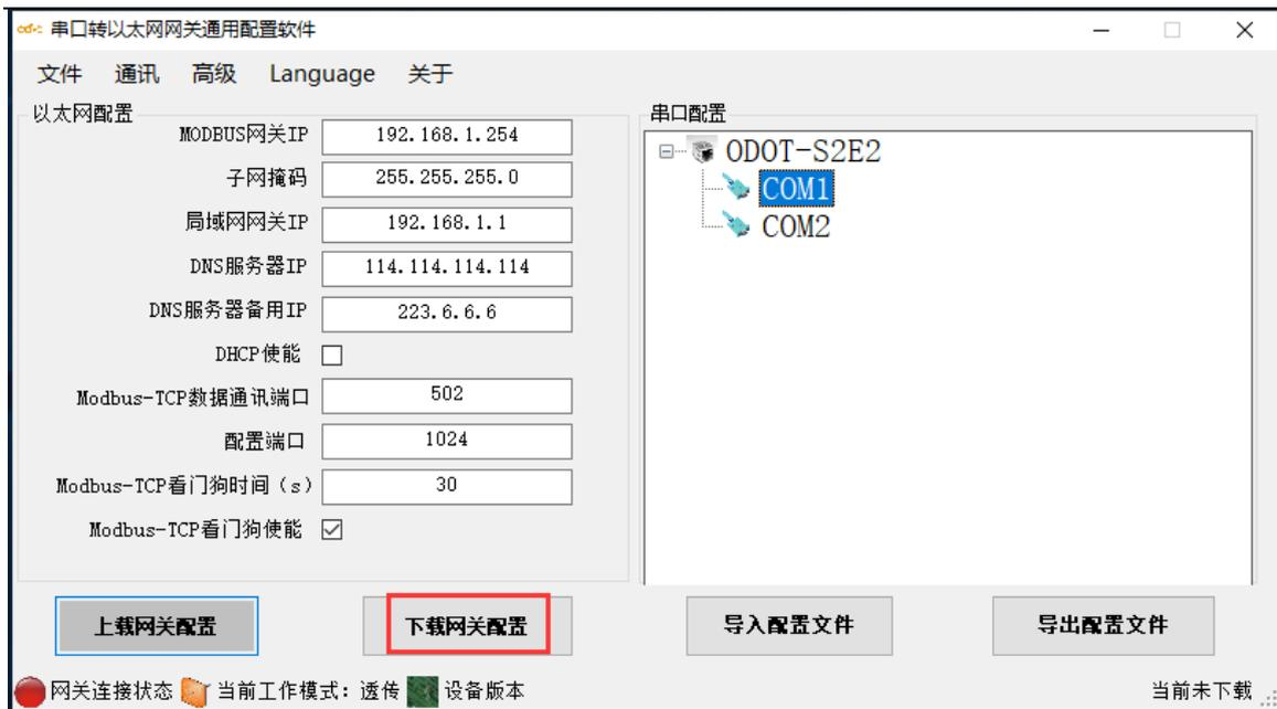
Figure 3.29 Download gateway configuration
