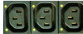
Example PDU with integrated Light Pipes
