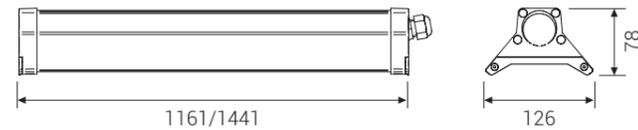
Fixture for continuous-row with quick connector and through wiring.
