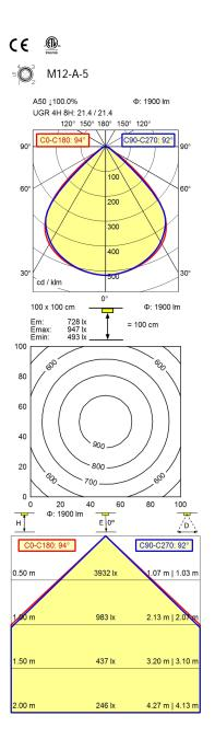
light source LED work equipment without connected load 24 V, DC env. 14 W power consumption luminous flux approx. 1.900 lm luminous efficiency approx. 136 lm/W light distribution direct 92° beam angle colour temperature neutral white colour temperatur approx. 5.000 K color rendering index (CRI) >= 80 chromaticity tolerance LED < 3 SDCM
