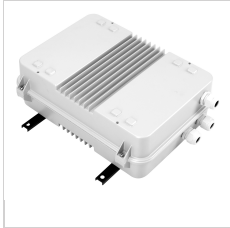
3105743 Drivers box 470 W - 1.1A - 2CH - DALI - 380-415 V 50/60 Hz Metallic grey
