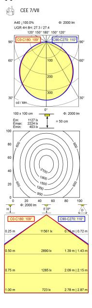
light source LED work equipment electronic transformer connected load 24 V secondary tension power consumption ca. 30 W sec. power consumption ca. 26 W
