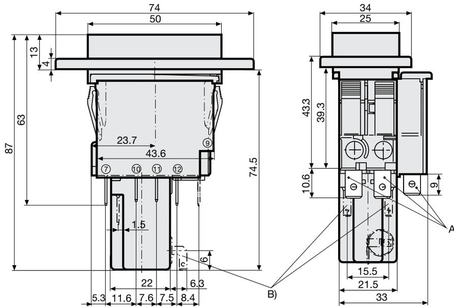
A) Quick connect terminal, IEC 61210, A6.3-0.8 mm
