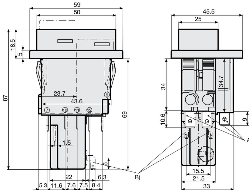
A) Quick connect terminal, IEC 61210, A6.3-0.8 mm
